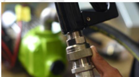
9. Attach swivel (and hose) to nozzle using provided Teflon tape.
