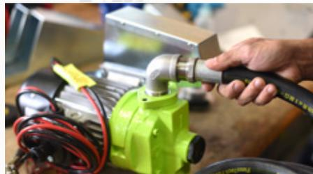
6. Connect hose to elbow using provided Teflon tape.
