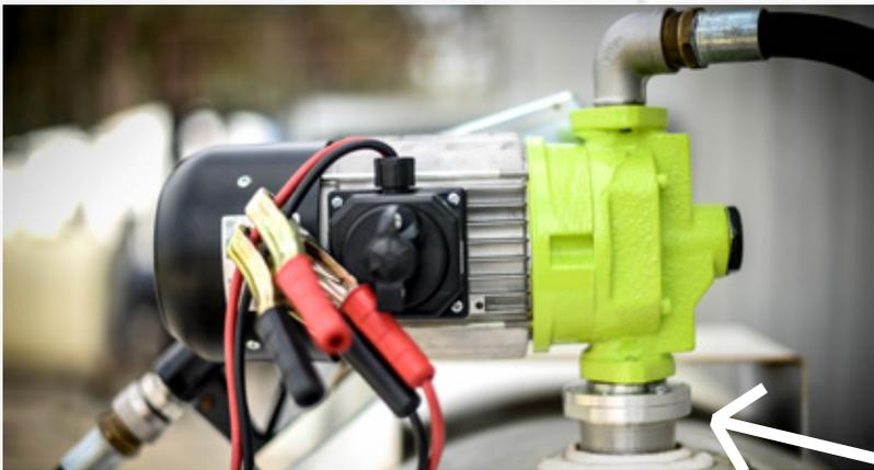
1. Screw provided adapter into 2" bung opening. Install downtube (not provided).
