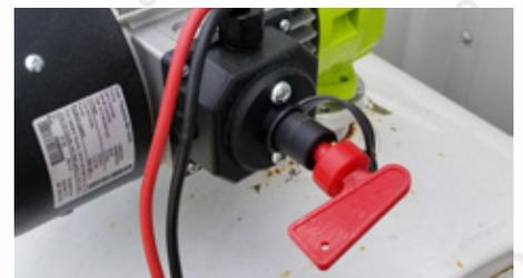
10. Use provided key (in red) to turn pump ON/OFF as needed.
