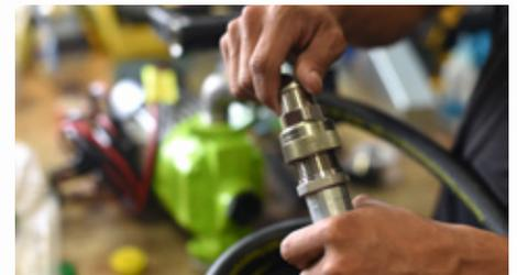
7. Connect swivel to opposite end of the hose using provided Teflon tape.
