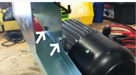
8. Attach nozzle holder to side of pump using provided bolts.
