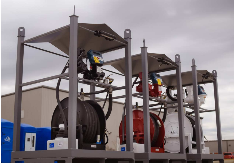
CUSTOM, MULTI-POINT MARINE FUELING SYSTEM
